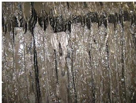
We decided to scrape samples off the RBC disk directly to see if the filaments were growing on the disks, or just in the screen and collection pit. We were quite surprised. Except for the areas where toilet paper and rags had collected on the disk and caused the biofilm to be trapped and turn older and septic, the majority of the biofilm was extremely young; amoebae and flagellates dominant. Floc was young, Zooglea was present.
