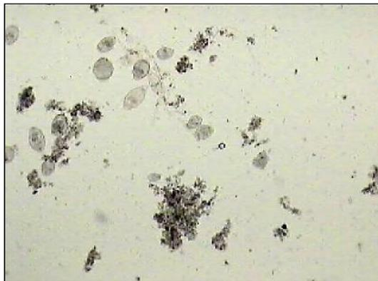
Section 1-Some filaments in areas, probably where fiber or debris and rags built up solids. Some areas with floc and stalks. Fiber and floc in section two. Amoebae and more single celled bacteria in section 3.
