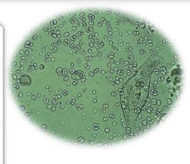
Plant loading seriously exceeded design capacity Foaming continual Tetrads and Type 021N filaments
