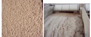
Foam due to M. parvicella - grease Foam due to septicity and 0914
