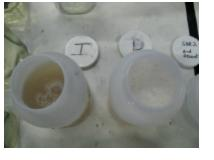
Bacterial activity is usually the main cause of foam in secondary treatment systems. This includes the production of surface-active decomposition products and gaseous fermentation of organic materials. Biological foam can be caused due to grease, septicity, low DO or just high BOD and very young sludge. Make sure you know what is causing the foaming, and it may be easier to change the cause than to use antifoams. Also antifoams do not work on every type of foam.
