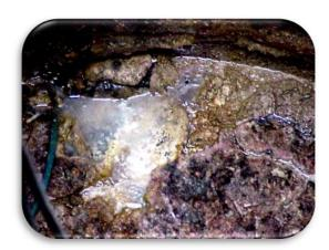
White milky water indicating bacteria is starting to work, cracks are starting to form in the grease; it is starting to soften and a little foaming is present.
